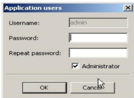
The password can be changed ( the default **password is 1234**). You have to enter the new password twice into the the two boxes and after that click on the **OK** button. You can add new users to the list as well. For example let the name of the new user be “user”. After that enter a password for this new user, twice.
