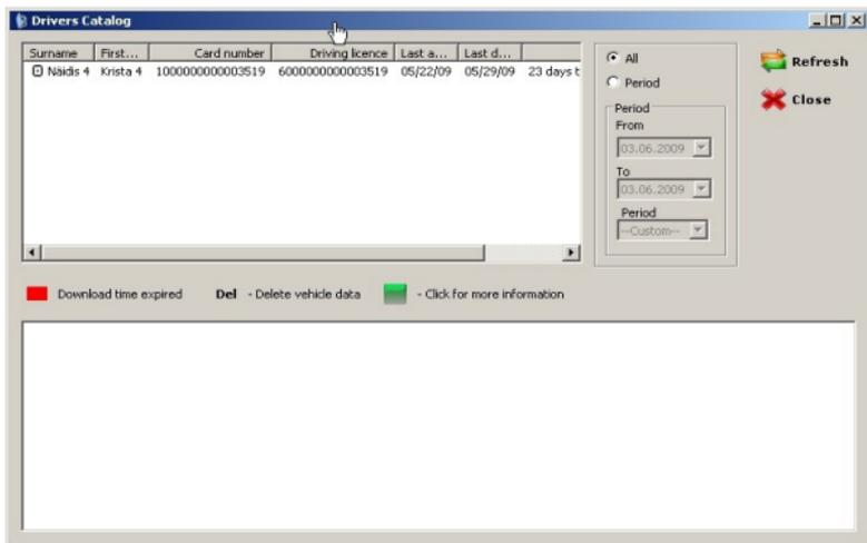
The list of the drivers is shown in the upper, left side of the window. All you need to do is click on the drivers name and it will turn blue. After that click on **Refresh** button on the right side. This operation can also be done by double clicking on the drivers name.
